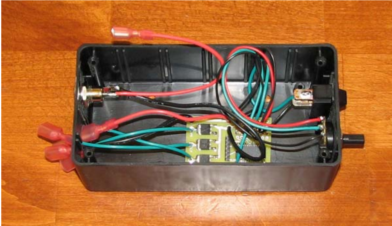
A plastic project box holds the MCU-and-FETs circuit board, a potentiometer, switch and connectors.
