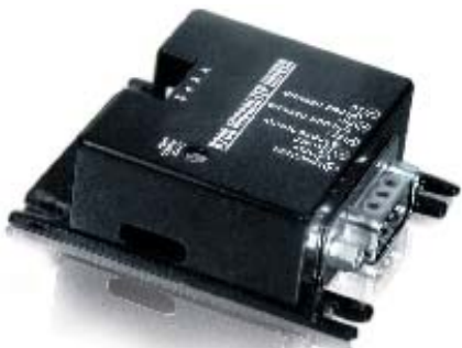
The R235 microstepping driver (top) produces 256x microsteps compared to the R208 that produces 8x microsteps.
