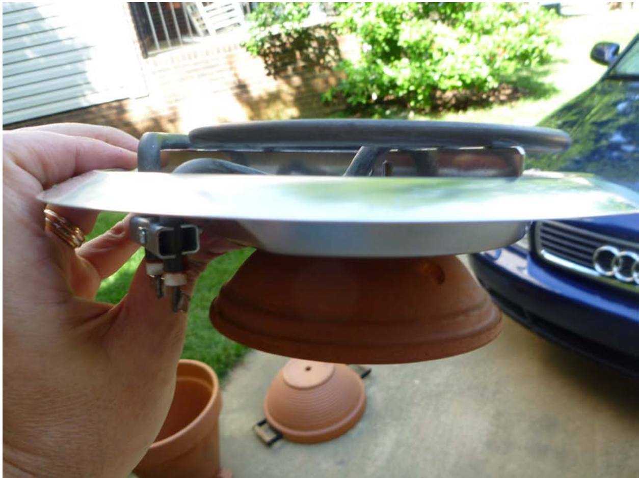
Figure 6. Hot-plate element attached to a terra-cotta base ready for insertion into the bottom of the smoker pot.
