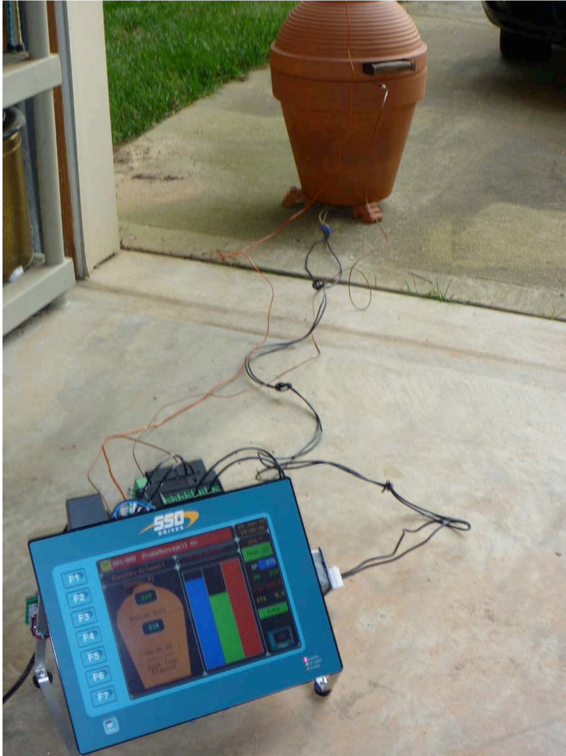
Figure 7. Smoker assembly in driveway with controller, HMI, and connections to thermocouples and the heater element.
