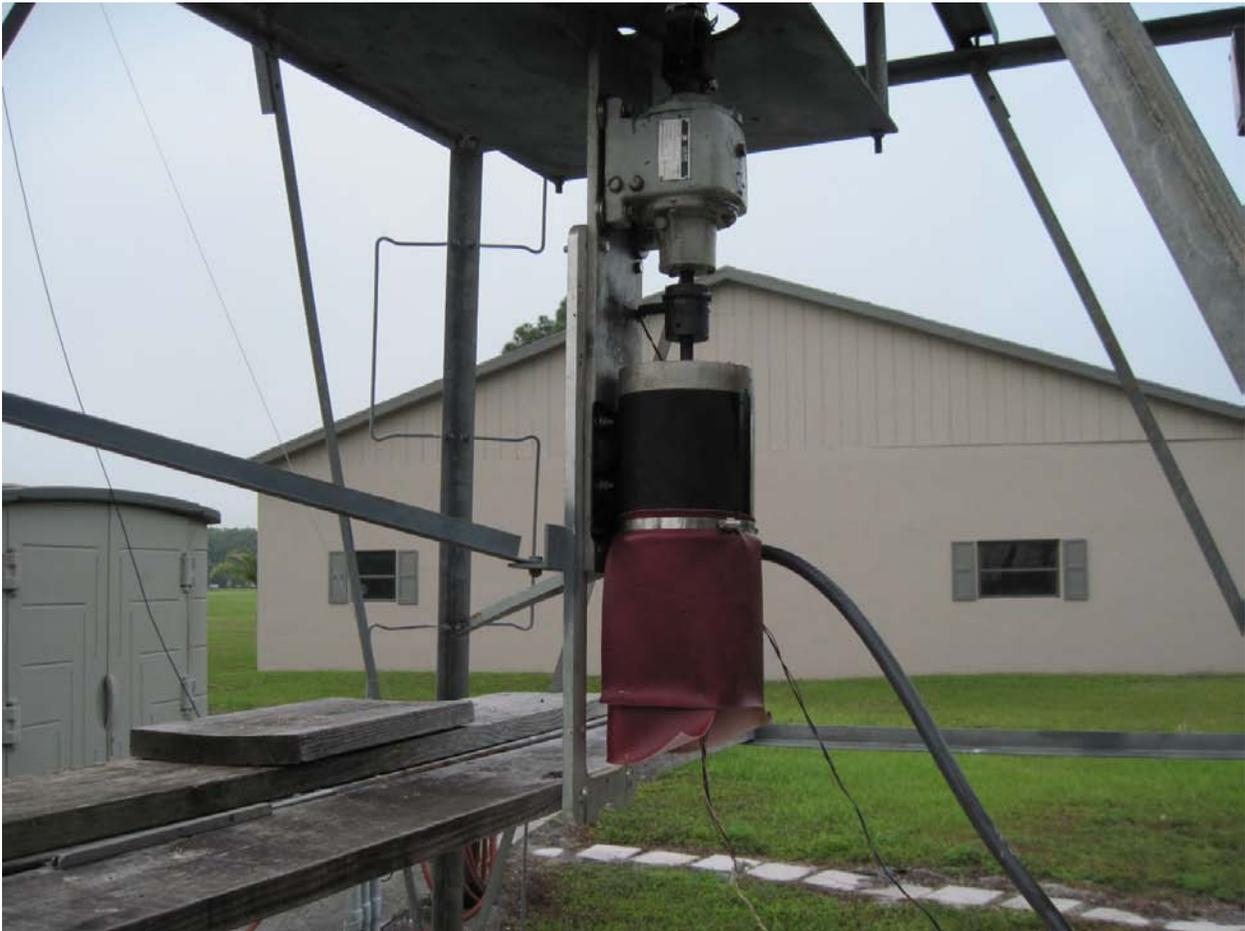
Figure 6. A "backwards" speed reducer (top, gray) provides power at 1800 rpm for the above the motor/generator (middle, black). The red rubber "boot" below the motor/generator shields the stepper motor used as a speed sensor.
