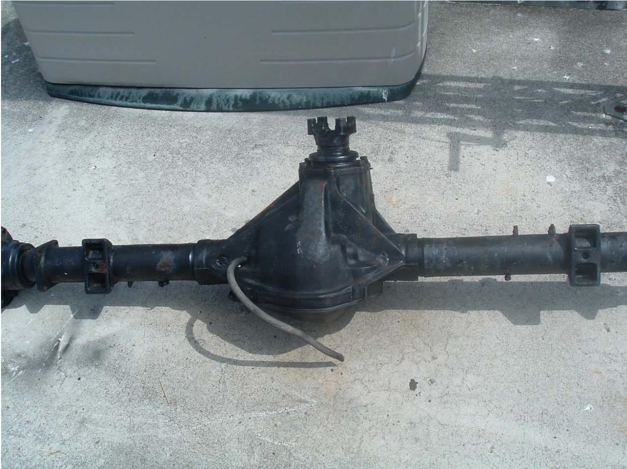
Figure 3. A wheel hub on this truck rear end, or differential, connected to the the rotating blades. The usual drive-shaft connection (upper center) connected to the long shaft that turns the motor/generator at the tower base.
