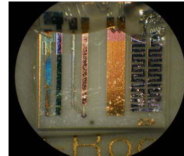
Multi-element sensor suite with MEMs viscosity Sensor
