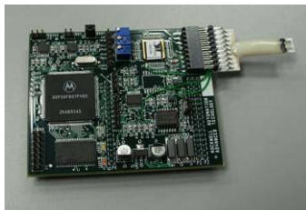
MEMs bio-sensor with interface board and sample sensor response in aging tomato liquid
