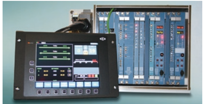
VPTC Onboard Computer and Locomotive Display Unit
